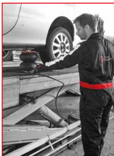
Balloon jack can be used on column lifts. Ideal for tire changing applications and bodywork shops
